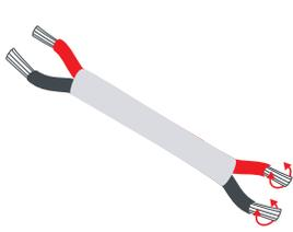
1. Cut a length of connection wire to run from Receiver to Tape Light location. Strip 1/4" insulation from both ends of wire, twist each wire, and fold stripped wires in half.
